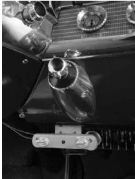
Toggle switches installed just below the dashboard near the steering column allowed Call to switch off the brake lights but leave the taillights burning if he were chased at night. That prevented the law from seeing where he was braking on the twisty roads of the North Carolina foothills.
