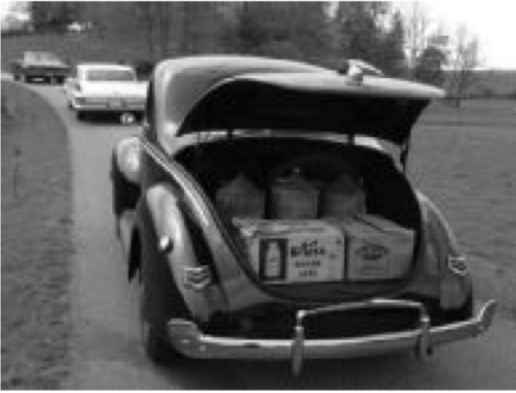
Equipped with extra-stiff springs to conceal the weight of the load, a '40 Ford could carry up to 22 cases of liquor, each holding 12 half-gallon glass jars of moonshine.
